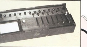
The Arithmometer. In 1820 the first commercially manufactured calculating machine was designed by a Frenchman, Thomas de Colmar, and some 1500 machines to his design were sold over a period of 64 years. The Arithmometer represented a great step forward, being capable of addition, subtraction, division and multiplication. Many variants of the machine were sold well into the century.
