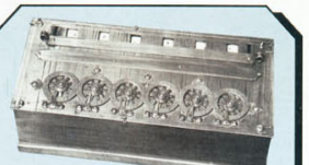
Pascal's Calculating Machine. The first calculating machine built to have a design in 1621 by Blaise Pascal, the French scientist and philosopher, invented his first calculator in 1642 and in just ten years he developed over 175 models capable of addition and subtraction. This picture of one of Pascal's machines shows the series of wheels carrying digits from 0 to 9, and the result windows similar to the display on a modern calculator.
